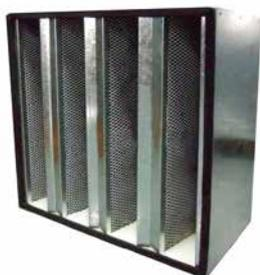
AC-VB is an activated carbon assembled in a galvanized steel frame and a rubber gasket on front side. This filter is filled with coal base activated carbon 4mm pallets characterized by their high adsorption capacity. It is used for the filtration of gaseous particles in application such as museum, archives or industry.
