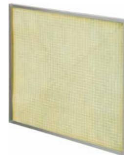
GPMC panel filter is constructed with a paint stop glass fiber media and assembled in a galvanized steel frame and a metal grid. It used as a prefilter for HVAC, industry and spray booth. This filter is available as ISO Coarse 50%.
