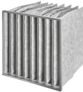
The HQ-AK is an activated carbon bag filter used for molecular filtration. It is assembled with a galvanized steel or aluminum frame and a high-loft micro glass fiber filtration media with activated carbon layer.
